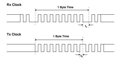
Times  $t_A$  and  $t_B$  vary as the clocks are adjusted to fit the exact byte periods of the target devices.
