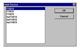
The Add Device window gives the user the choice of near and far devices. The user should select the required device form corresponding to the device located in the near or far signalling processor board. Finally, click on the OK button.
